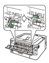
Open the back cover of the printer and make sure the two green envelope levers on the right and left hand side are in the up position. Close the back cover.
