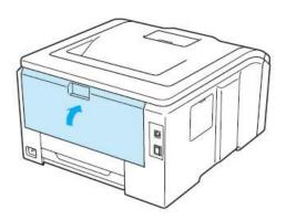
If you print the envelope or thicker paper, change the both lever position to the envelope one, and then try to print again with the back cover opened.
